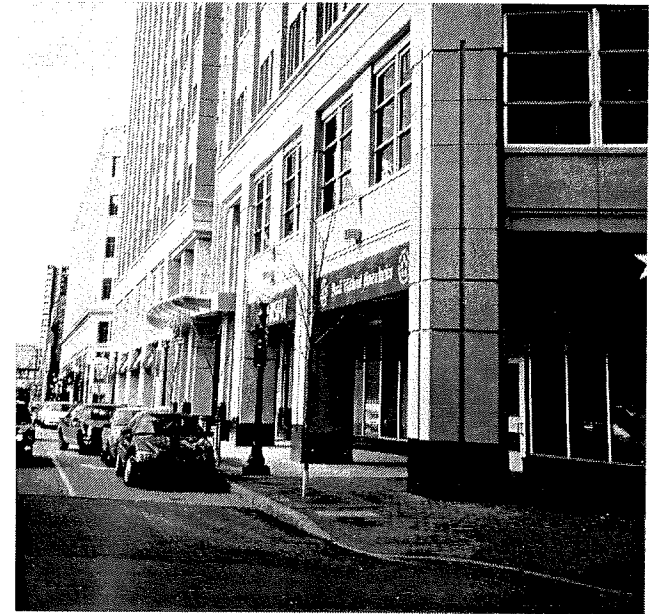
On-street parking can improve pedestrian safety by providing both a buffer between the pedestrian and traffic, and by adding "eyes on the street."
